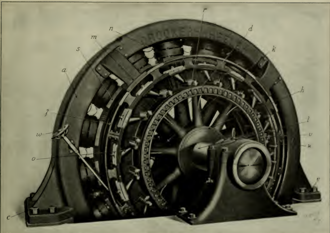
FIG. 302. LARGE DIRECT-CONNECTED GENERATOR BUILT BY THE CROCKER-WHEELER COMPANY
